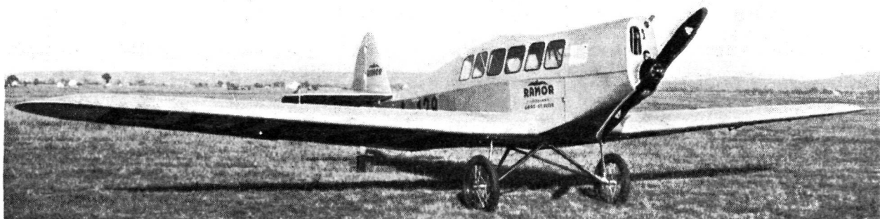
25 H.P. PER OCCUPANT: This Austrian Ramor K.E.14 carries four people on a de Havilland "Gipsy I" engine.
